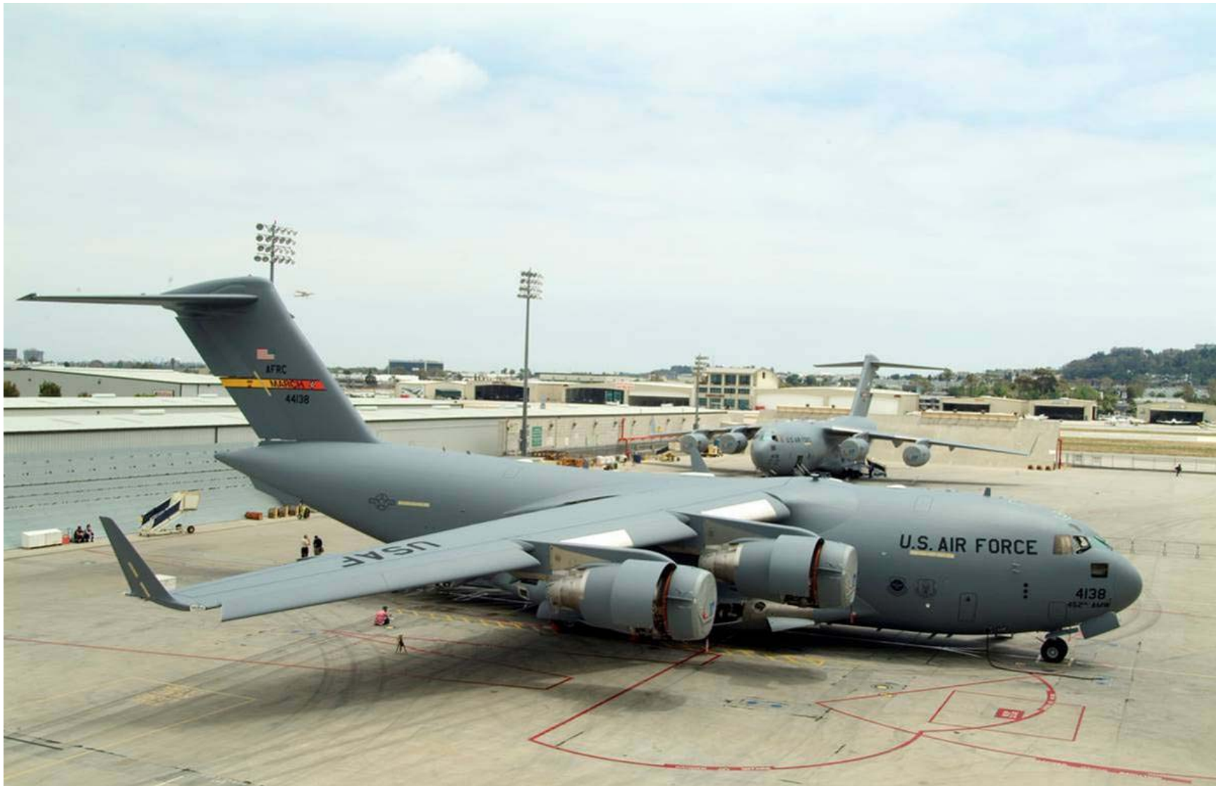
Completed C-17 Globemasters, each fitted with four Pratt & Whitney F117-PW-100s engines, stand ready for delivery to the U.S. Air Force.
