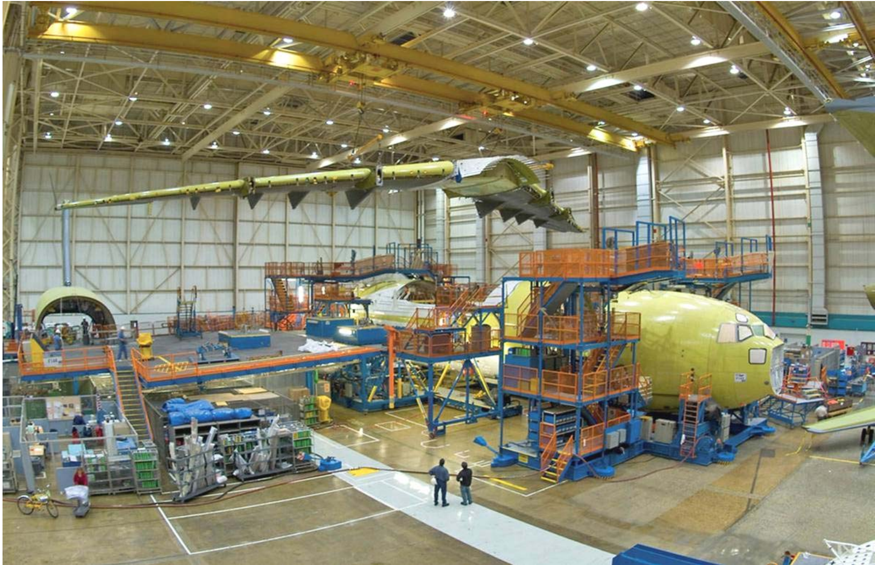
Massive C-17 wing assemblies are lowered by crane on top of aircraft fuselage sections where they are joined together.
