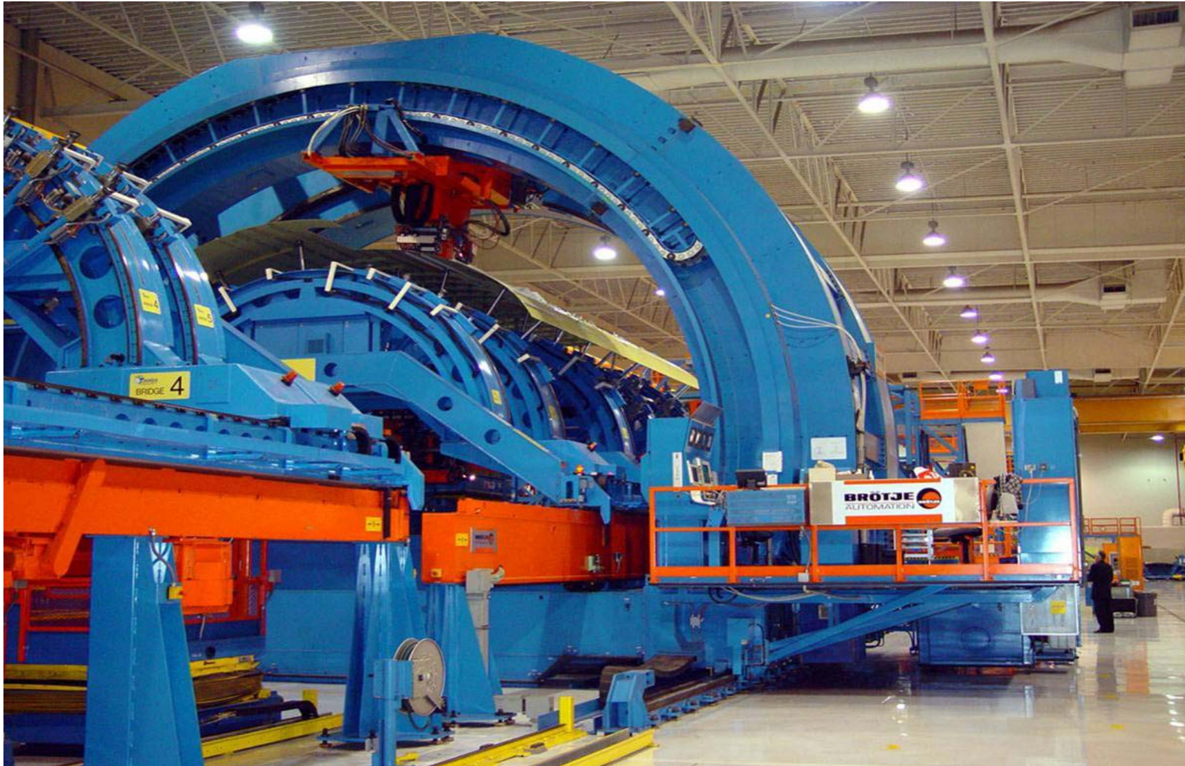
C-17 fuselage units are assembled using a massive custom automatic-riveting machine, which fastens aircraft skins to the fuselage frame.
