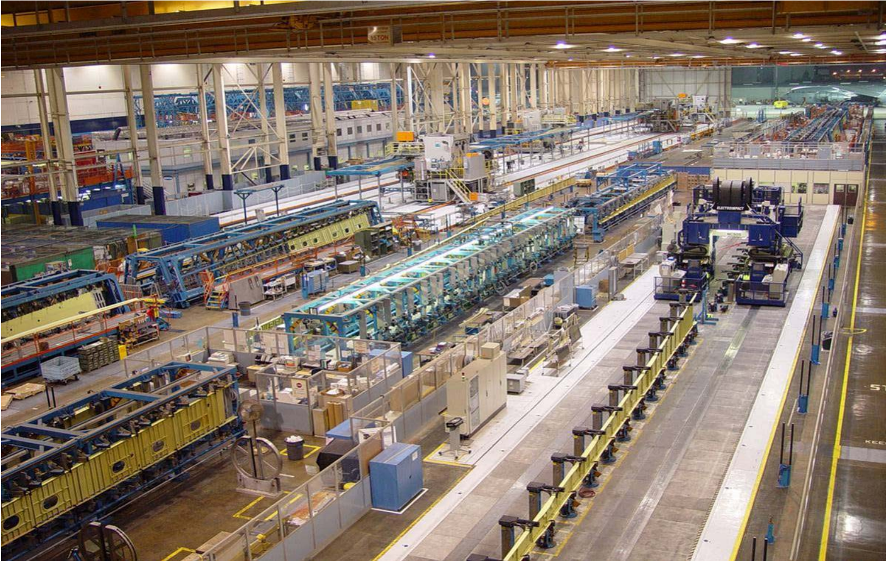
Construction of gigantic C-17 wing units requires the use of numerous high-precision jigs, alignment tools, and fastening systems.
