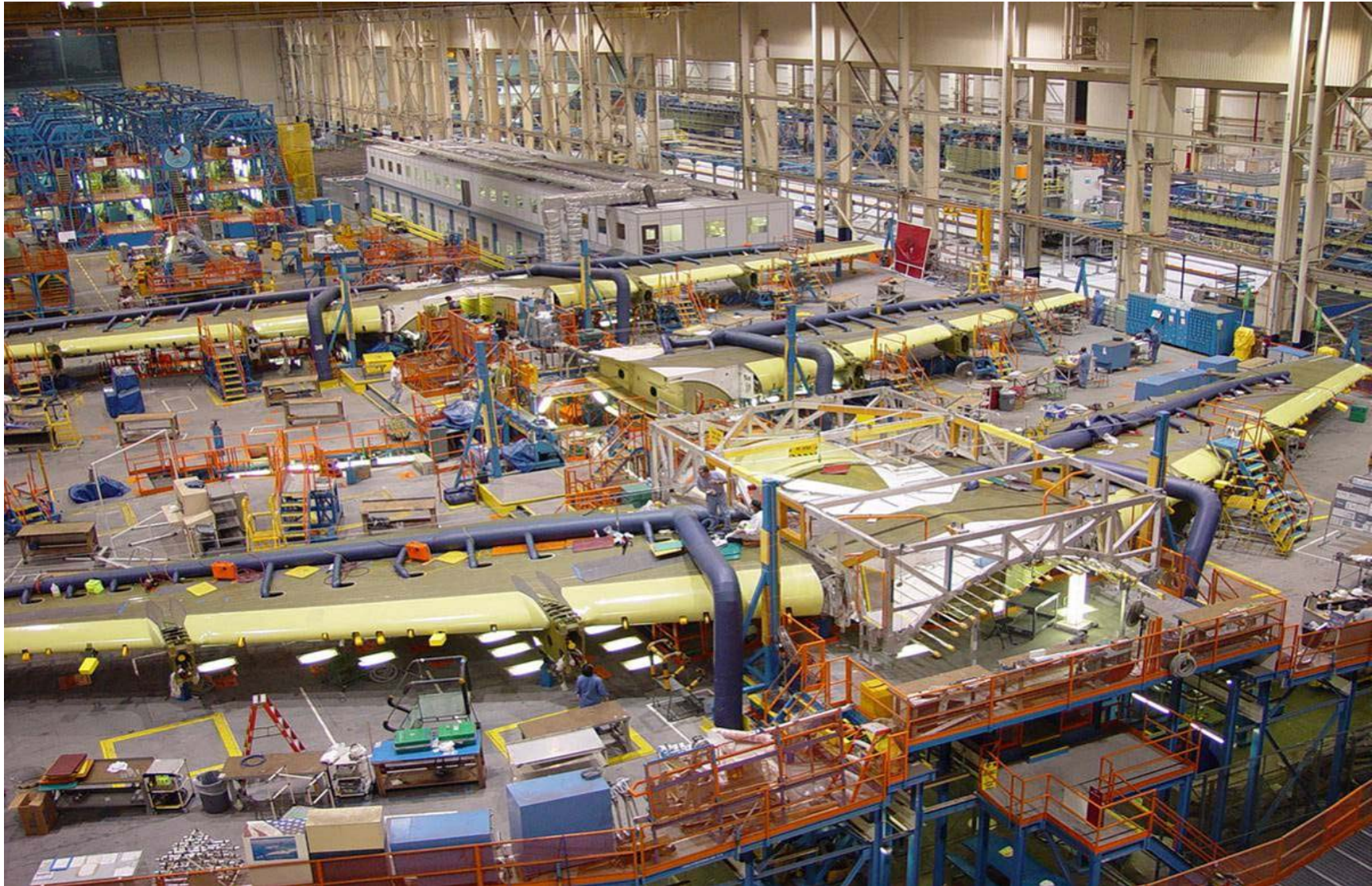
C-17 wing assemblies, including controls, fuel cells and engine pylons, are being prepared and tested prior to being mated to the fuselage.
