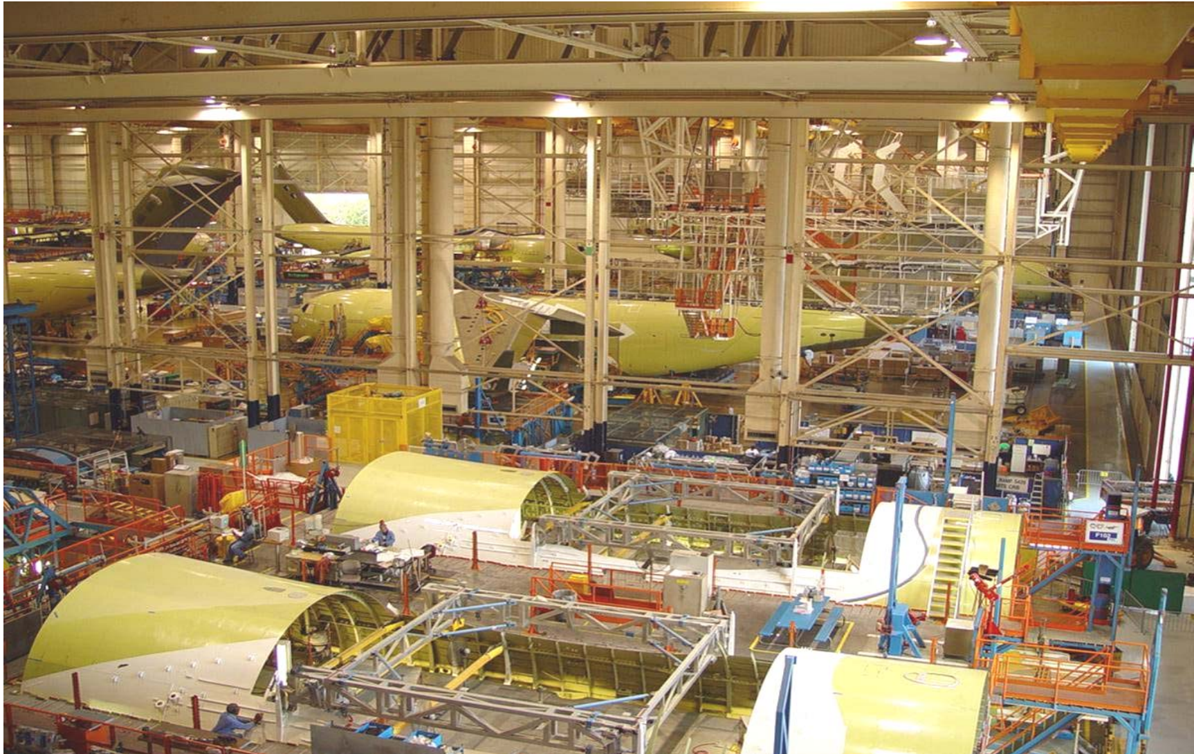
C-17 Fuselage sections (foreground) stand in assembly jigs in preparation for being joined together with other sections at Long Beach, CA.
