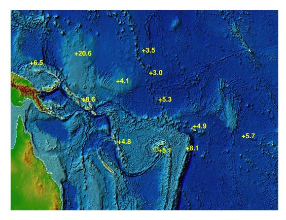
Figure 16. The net relative sea level trend in mm/year after subtracting the effects of the vertical movement of the platform and the inverse barometric pressure effect utilising all the data collected since the start of the project up to the end of June 2009.
