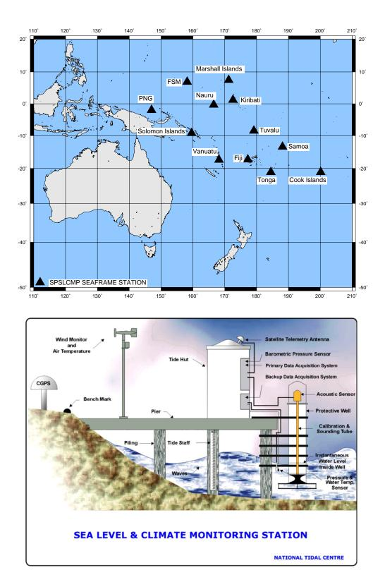
Figure 1. South Pacific Sea Level and Climate Monitoring Project sites (top) where sea level and climate monitoring stations (bottom) are installed.
